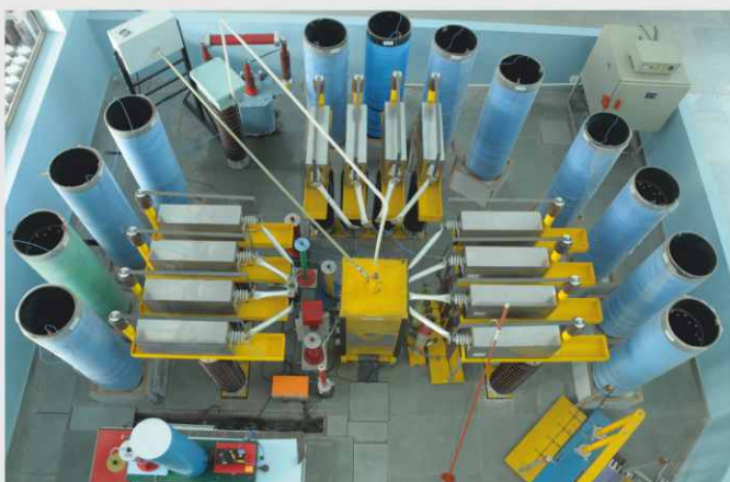
150kA Current Generator
